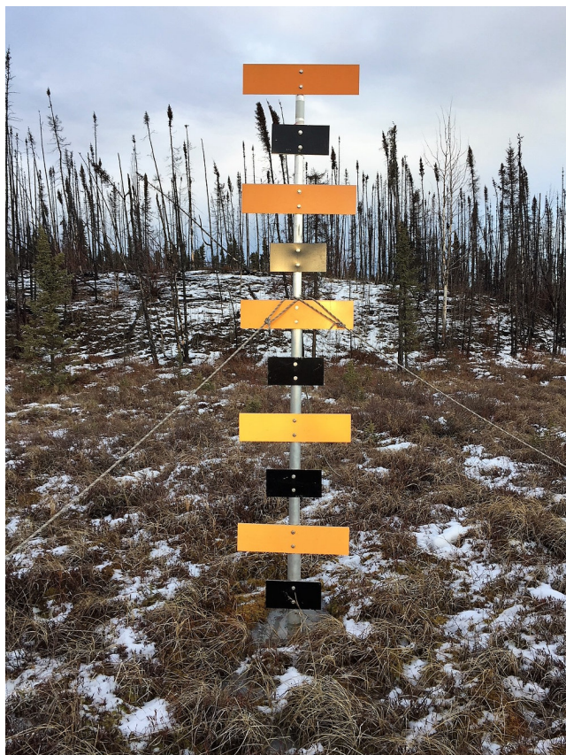
One of the aerial markers used to monitor snow depth on the Kenai National Wildlife Refuge.
