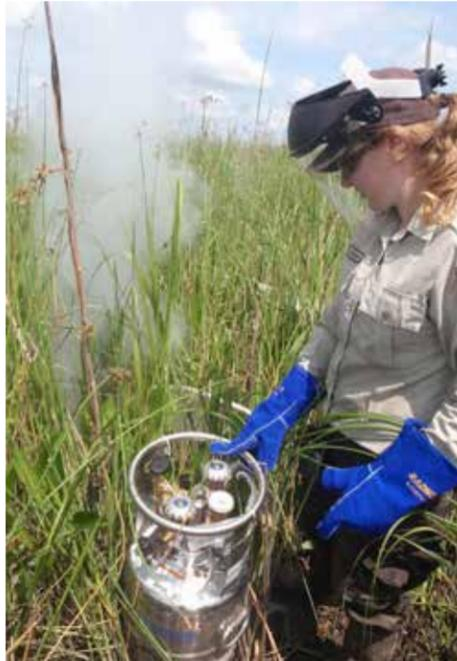
Nicole Rankin uses the cryogenic coring method to collect a sediment core from ACE Basin NWR, credit USFWS/Theresa Thom.
