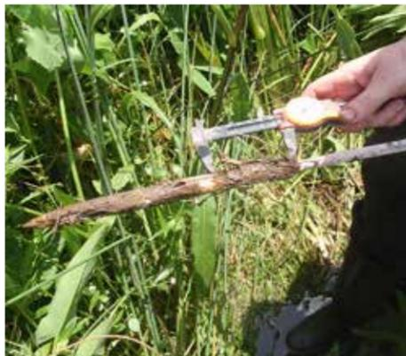
Sediment deposit on feldspar layer at Waccamaw NWR is measured from a cryo-core, credit USFWS/Theresa Thorn.
