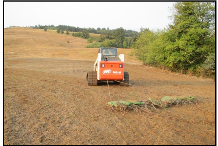
Figure 5. Refuge staff preparing the ground for seeding using a chain drag harrow to break up rhizome mats. Photograph by IAE.
