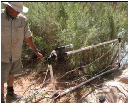
A submersible Passive Integrated Transponder tag antenna constructed by Marsh & Associates, LLC was installed in the Little Colorado River in April. The antenna has been continuously contacting tagged fish throughout April and May.
