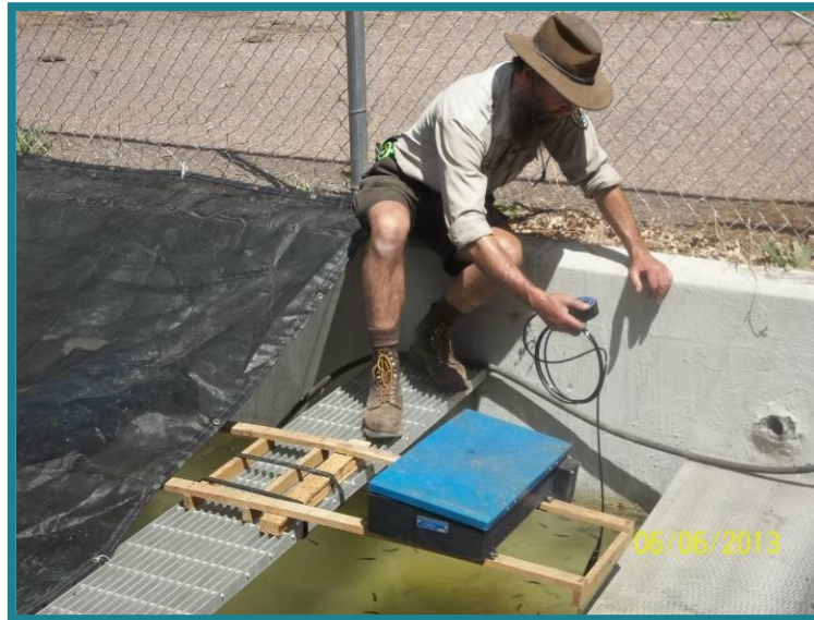
Dan Ragen using the new OxyGuard meter to measure dissolved oxygen and total gas saturation on A1 raceway at the Williams Creek Unit prior to an Aquaflo treatment
