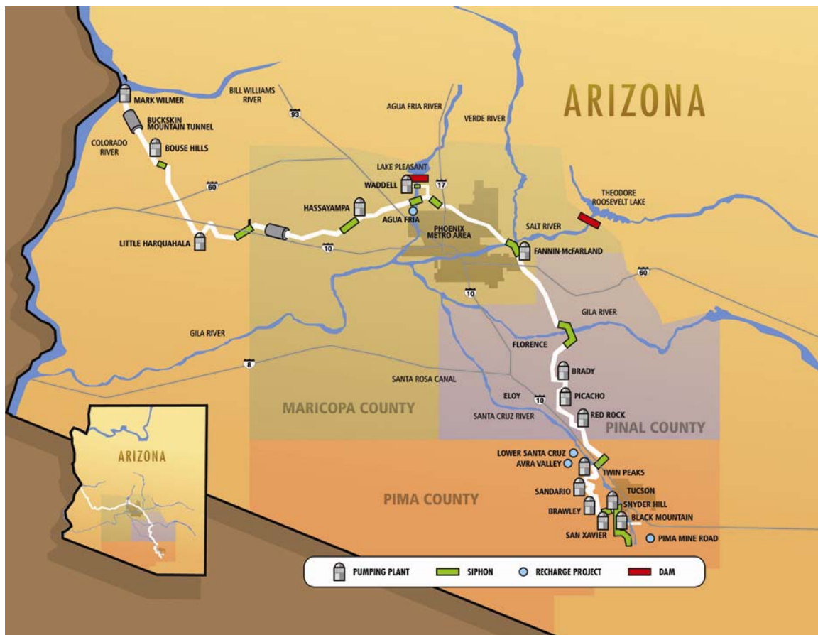
Figure 1. Map of the Gila River basin, showing major rivers and the route and primary features of the Central Arizona Project canal.
