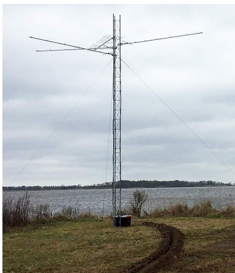
Automated radio telemetry station (Motus station) at Mackay Island National Wildlife Refuge, North Carolina, credit USFWS/Adam Smith.
