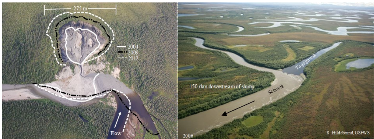
Figure 2.—Aerial views of the permafrost thaw slump in the upper Selawik River drainage and its erosion progression 2004–2012 (left image), and at the confluence of the Selawik and Tagagawik rivers in 2006 (right image), approximately 150 rkm downstream from the slump, illustrating the persistence of the turbid flow.
