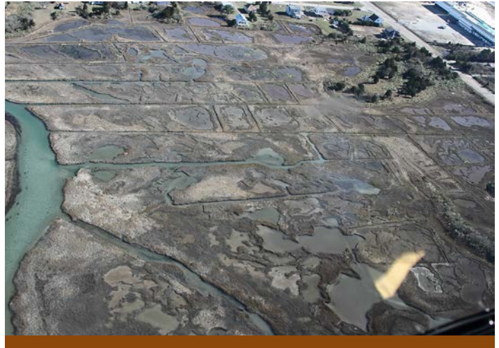
Historic ditches exacerbate flooding and reduce marsh integrity (Winnipaug Marsh in Rhode Island). USFWS
