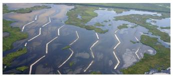
Duck-wing shaped terraces reduce water turbulence and encourage plant growth.
