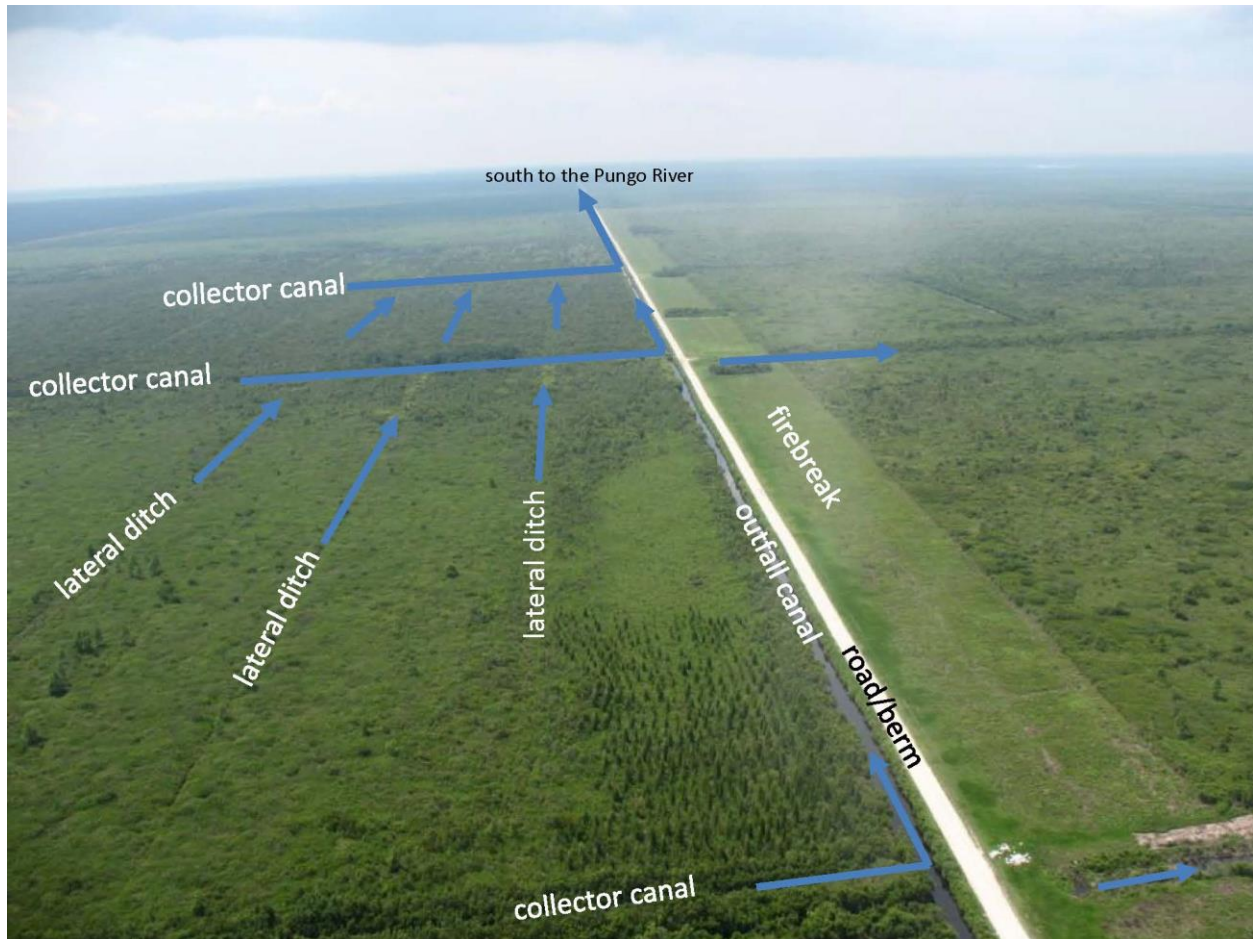
Figure A-24. Rainwater drainage through outfall and collector canals and lateral ditches.
