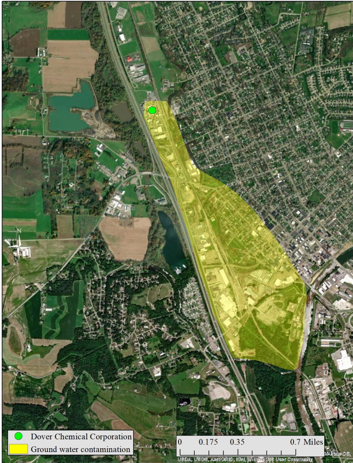
Figure 1.2: Approximate extent of ground water contamination within the Sugar Creek buried valley aquifer and the approximate area where ground water injury was assessed based on the extent of contamination within the Sugar Creek buried valley aquifer that extends approximately one and one-quarter miles south of Dover Chemical Corp. and encompasses approximately 174 acres.
