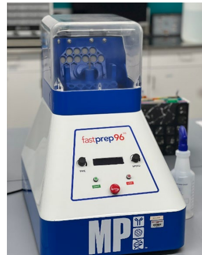
Figure 13: The sample prep machine is the MVP of WADDL's Aquatic Health Laboratory during peak ELISA season. It homogenizes samples by shaking beads at 10,000 strokes per minute.
