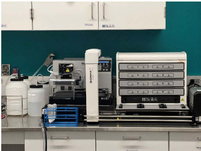
Figure 14: The ELISA Robot. Each of the 8 drawers on the right can incubate an ELISA plate under the specific conditions needed for each step in the assay. To the left is a robot that can remove plates from the incubator, wash them, add new reagents, put them back into the incubator, and then send them to the plate reader when they are done.
