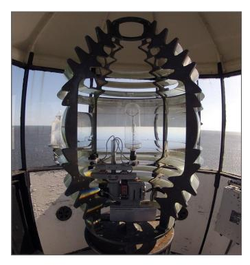
Our Fresnel (fre-NEL) lens, invented by French physicist, Augustine-Jean Fresnel, was installed in 1867 when repairs were made to the lighthouse after the Civil War. The lens, a Fourth Order fixed light, is constructed of various-sized prisms which gather light from a weak source and project a strong, steady beam. *St. Marks Refuge files*
