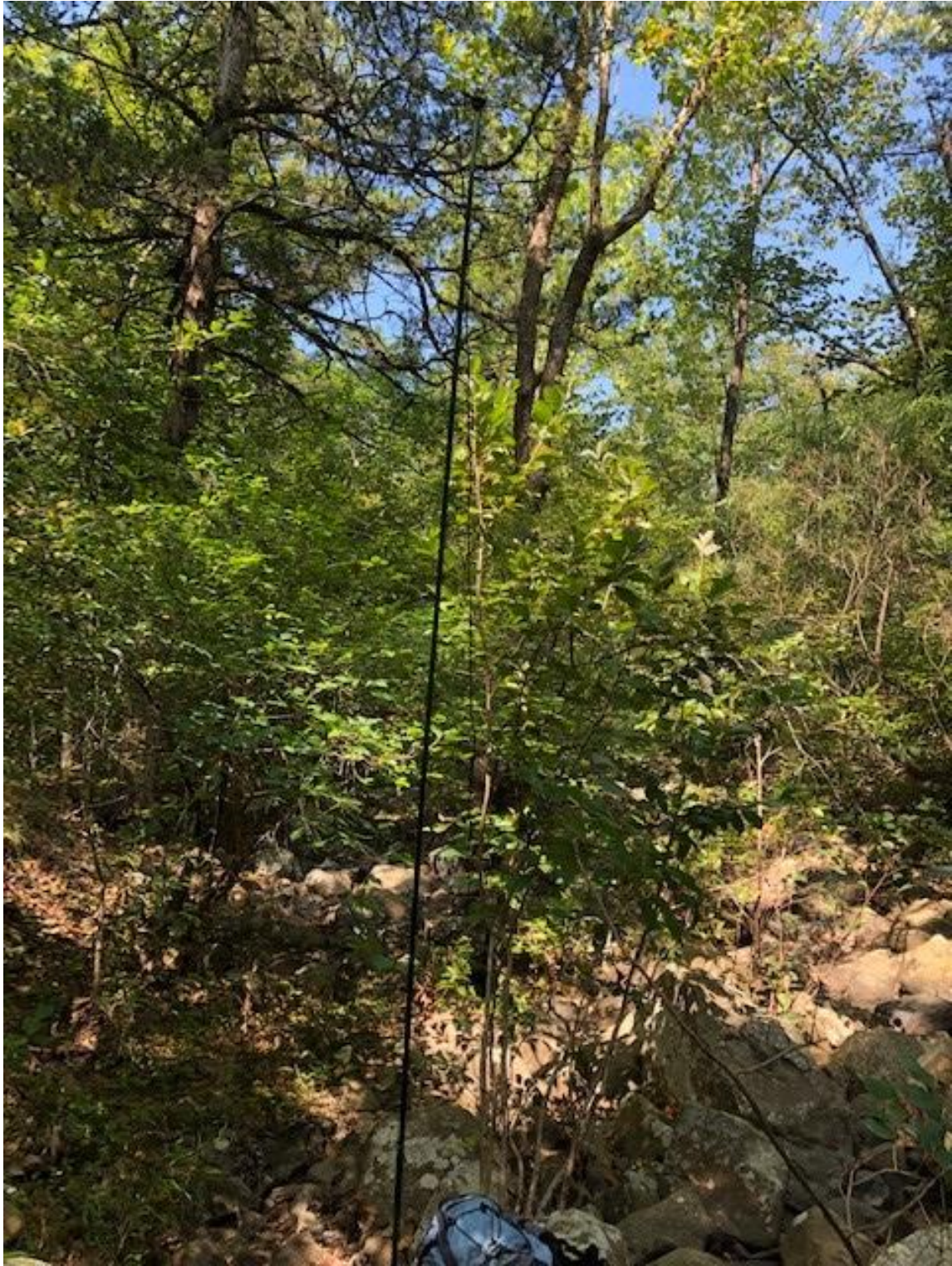
Figure 3. ANABAT Express at Jackson property site 2 with omni-directional microphone, detached and elevated by extension cable 4m above ground and positioned to record horizontally into a high, closed canopy.
