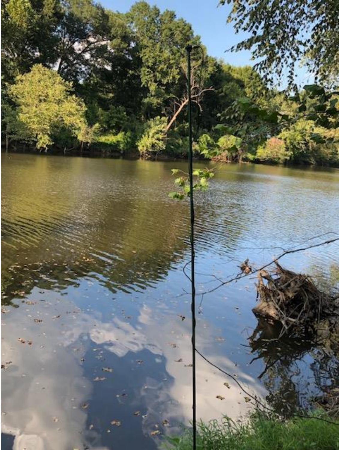
Figure 2. ANABAT Express at Jackson property site 1 with omni-directional microphone, detached and elevated by extension cable 4m above ground and positioned to record horizontally across the Kiamichi River in Pushmataha County, OK.
