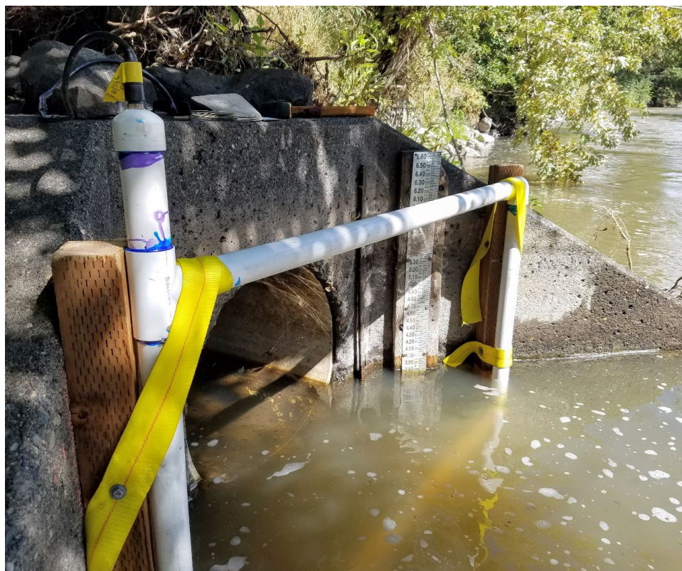
Figure 4. Fixed PIT antenna at the bypass outfall of the Feed Diversion Canal.
