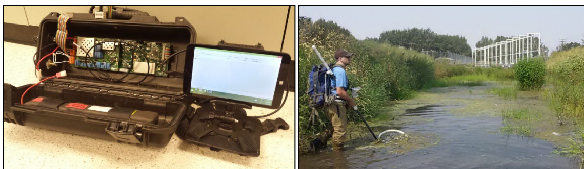
Figure 7. An IS1001ACN-based mobile PITpack reader system. (A) The PITpack reader is comprised of a waterproof Pelican case, a Windows-based tablet mounted in a harness, a detection alarm, and a lithium-ion battery. (B) Scanning a drained Feed Diversion Canal
