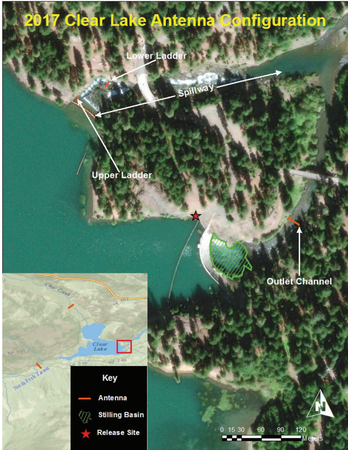
Figure 6. Map of the area around Clear Creek Dam on the NF Tieton River, Yakima County, WA. Shown on the main map are key areas and the location of the PIT tag detection antennas around the dam. The inset shows the location of the dam on Clear Lake as well as the PIT tag detection arrays in Clear Creek and the NF Tieton River.
