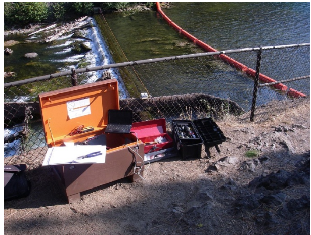
Steel job box holding batteries and tag readers
