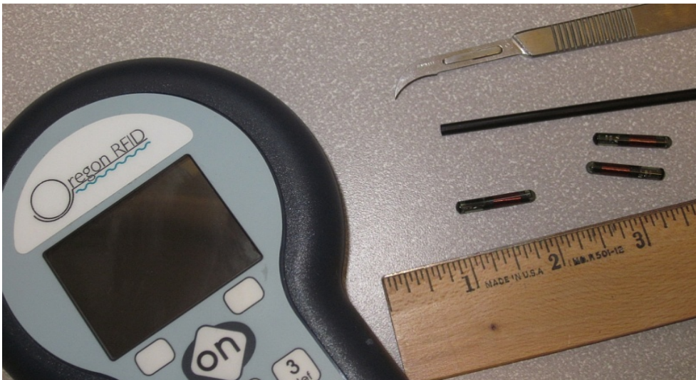
HDX PIT tags, scalpel, insertion straw and Oregon RFID® portable tag reader
