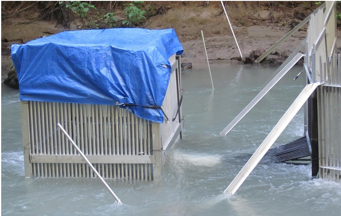
The modified configuration of the trap used in 2013. Note the modified entrance leading to the PVC pipe extending into the trap. The trap itself sits about five feet from the entrance.
