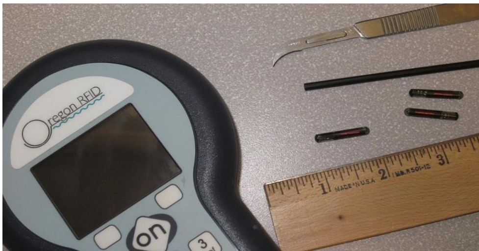
HDX PIT tags, scalpel, insertion straw and Oregon RFID® portable tag reader
