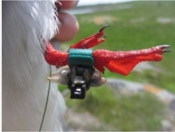
A geolocator, wrapped in a waterproof cover, attached to the leg of an Arctic Tern
