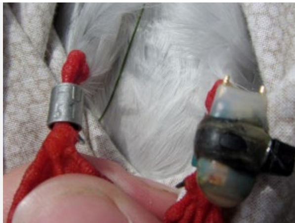
A geolocator (right) and a field-readable band (left)
