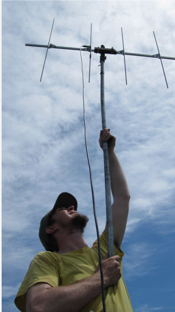
Increasing antenna height even a few feet can tremendously help signal reception.
