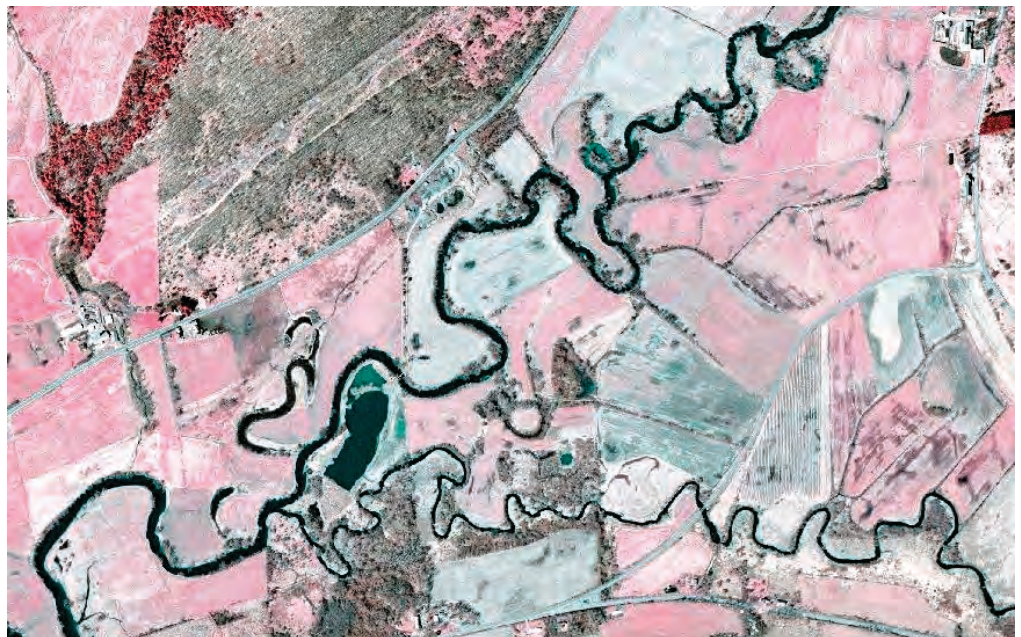
The looping pattern of a river or stream is called a meander. These bends result in a longer channel with a lower slope. (Aerial photograph by NYS Office of Technology and Cortland County.)
