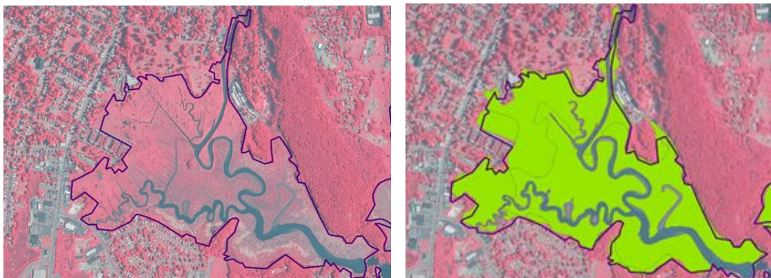
Figure 4. Example of 1970s (left) and 2000s (right) wetland data for Connecticut; note the inclusion of hydrographic features as part of the 1970s polygon (left) and the exclusion of hydrographic features in the 2000 era NWI emergent tidal wetland data (right, only green area is counted).
