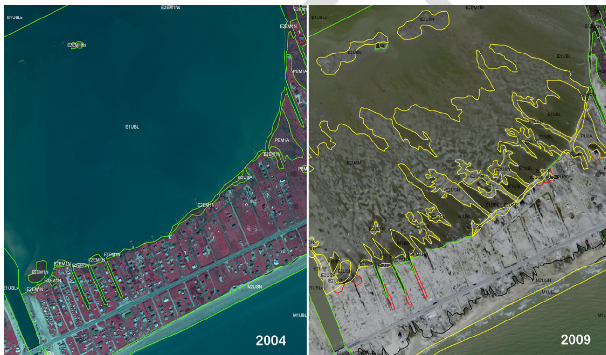
Figure 9. Extensive storm damage from Hurricane Ike, Rollover Bay, Bolivar Peninsula. Green lines indicate existing wetlands; red lines are wetlands lost to upland, black lines are wetlands gained from upland, yellow lines are converted wetland types.
