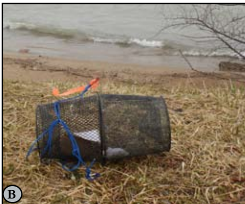
Due to heavy wave action causing damage to several traps (A), survey methodologies were modified and incorporated sturdier, metal traps (B).
