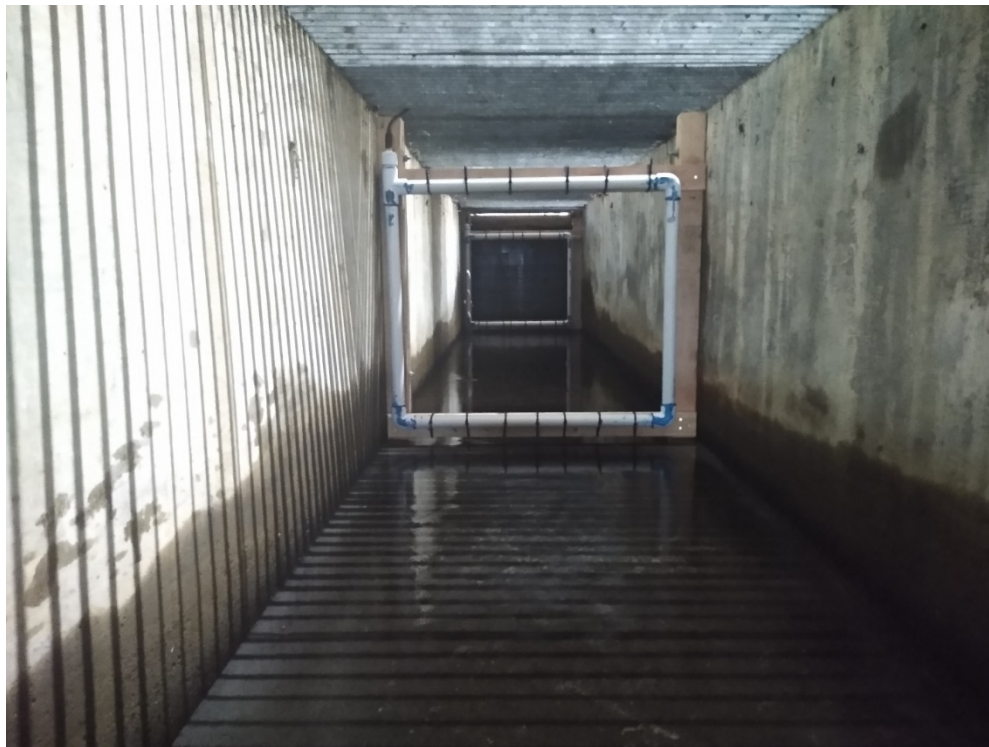
Figure 5. FDX PIT tag antenna array located in secondary bypass channel, immediately downstream from sampling Unit 1.
