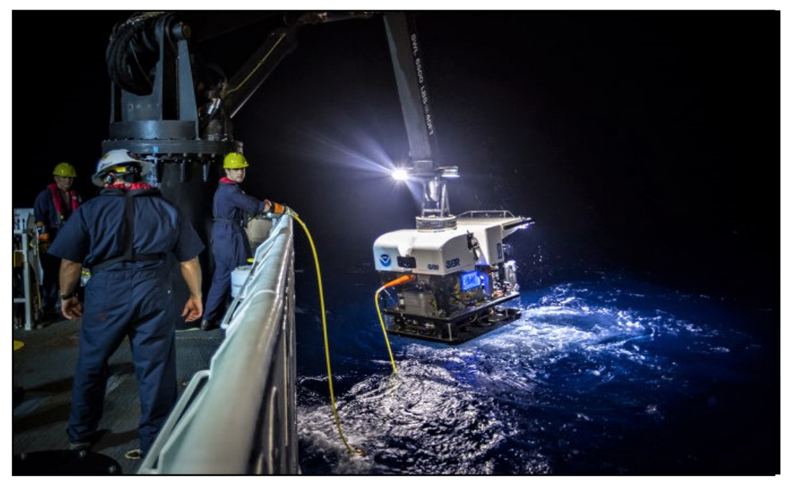
Recovering remotely operated vehicle Deep Discoverer . NOAA OER 2016 Deepwater Exploration of the Marianas.
