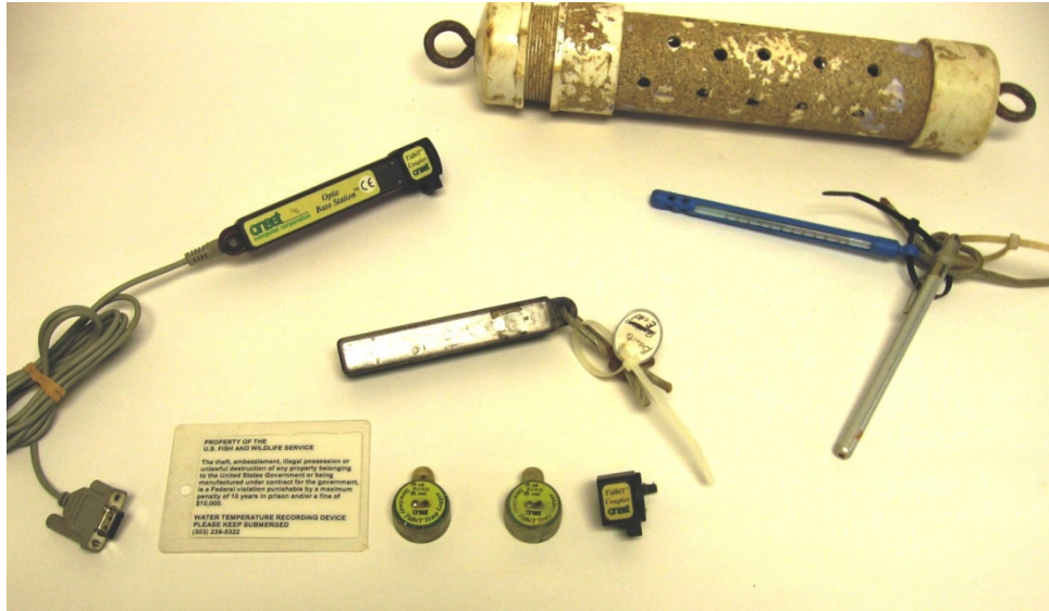
Figure 3. A collection of stream temperature logging and reading devices used by the Program over the decades. Over time, devices that were originally large and bulky (top) evolved to become increasingly more reliable and compact, culminating in the current compact tidbit technology (bottom center).
