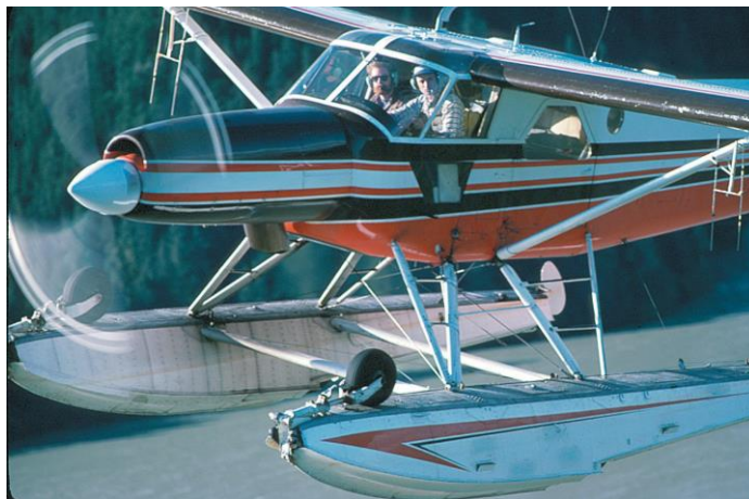
N-754's distinctive nacelle (engine housing) contains a Garrett turbine engine
