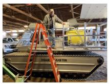
The Marshmaster was recently upgraded with passenger rails and seats. Gary Galvagni, of Industrial Sheet Metals, provided the upgrades to the machine. The Marshmaster is used for habitat management activities, including invasive plant control and controlled burns, and is designed to operate in wetlands and marshes.
