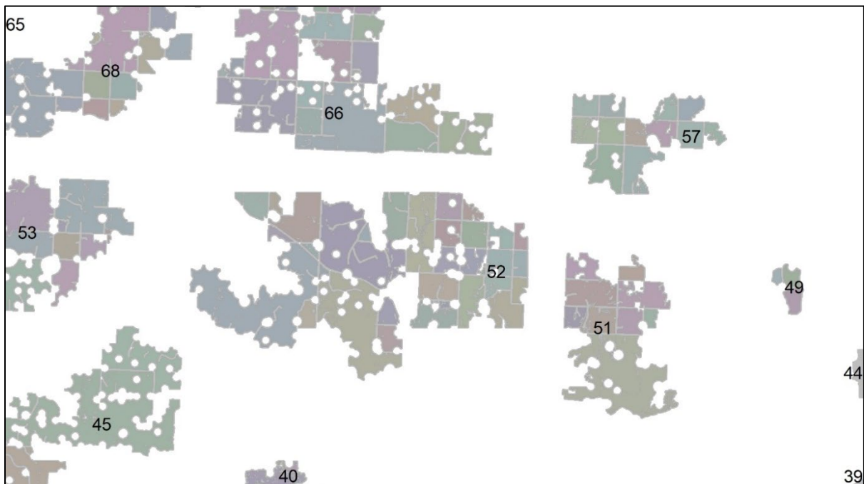
Figure B.14. Steps 2 and 3. A 70-meter buffer polygon layer (gray transparent) is created from every polygon (buffer layer is a separate Feature Class). All separations less than 140 meters are now removed in the Buffer Layer. Each buffer polygon has a unique number (from the Buff_ID field).
