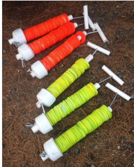
Figure 6. Painted steel washers marked the start (green [lower three stacks], downstream) and end (orange [upper three stacks], upstream) of the polygons.
