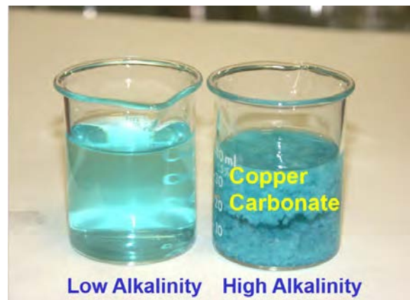
Figure 12: The chemistry of copper sulfate (used to control parasites in pond aquaculture). When alkalinity is low, copper stays in solution and is very toxic. At high alkalinity it precipitates out as copper carbonate so quickly that parasites are not killed.
