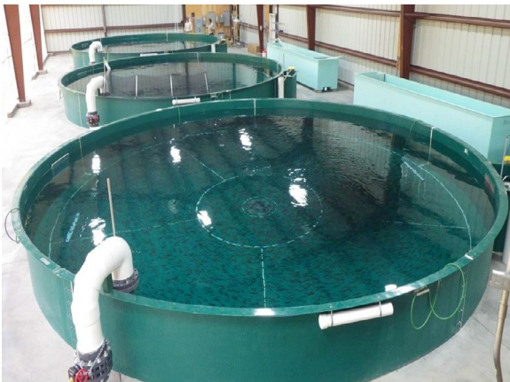
Figure 14: Managing water speed in pRAS systems is critical. If speeds are too high the fish are stressed by overexertion and infectious disease outbreaks occur.
