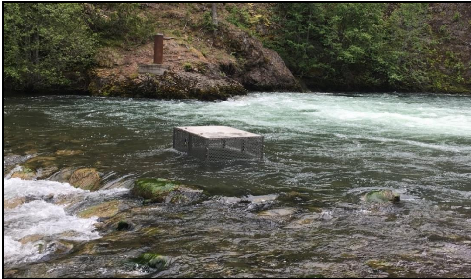
Figure 1. Stainless steel pen (0.9 m x 1.2 m x 1.8 m) used for holding Bull Trout after collection and before rapid response genetic testing and transport.
