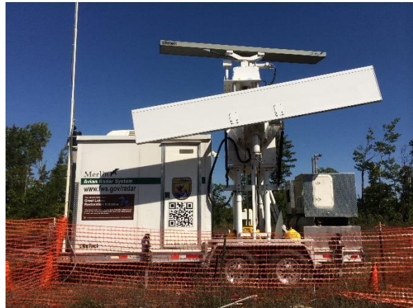
A Merlin radar system, with horizontal and vertical antennas, used to track migration movements.
