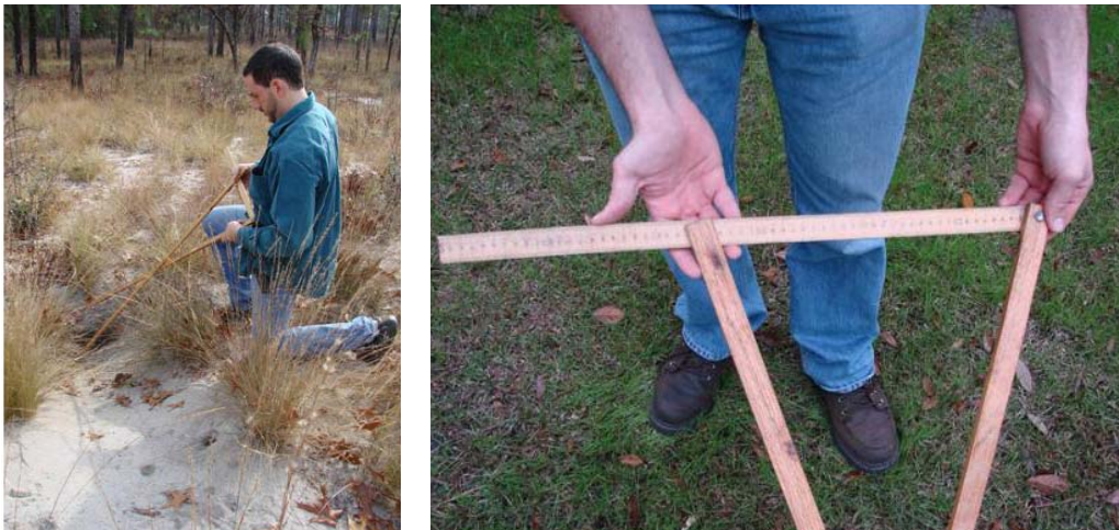
Figure 6. Use of calipers to measure the width of a gopher tortoise burrow. Measurements should be taken in metric units (mm or cm) at 50 cm inside the burrow entrance.
