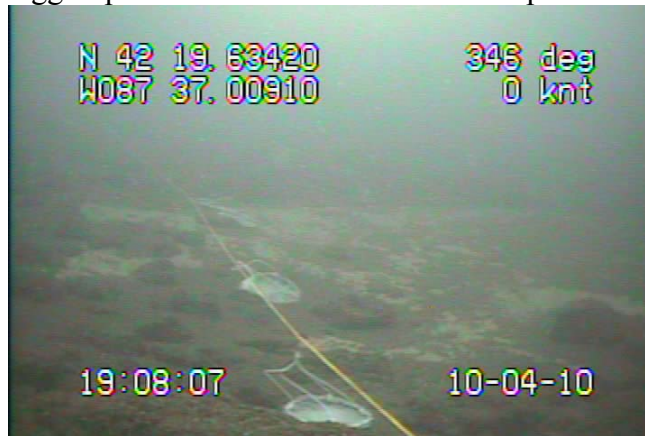
Figure 21. Deep-water egg traps on lake bottom shortly after deployment at Waukegan reef during the 2010 lake trout spawning season.
