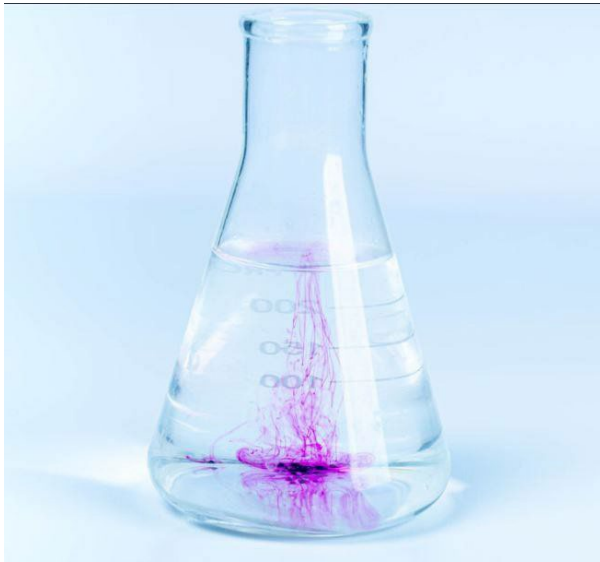
Figure 22: Potassium permanganate in water. It is purple when it is still an active oxidizer and brown when it is used up.
