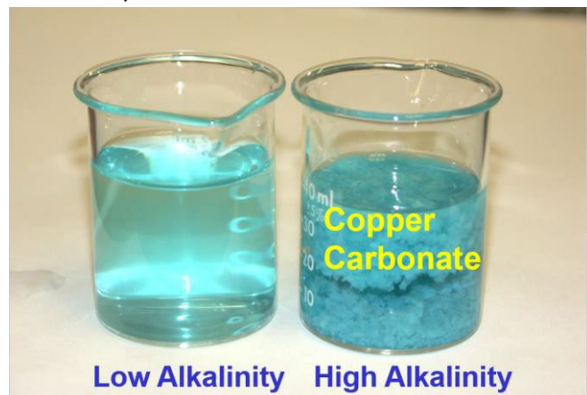
Figure 23: Copper sulfate in solution (left) and as a copper carbonate precipitate in water with high alkalinity (right).
