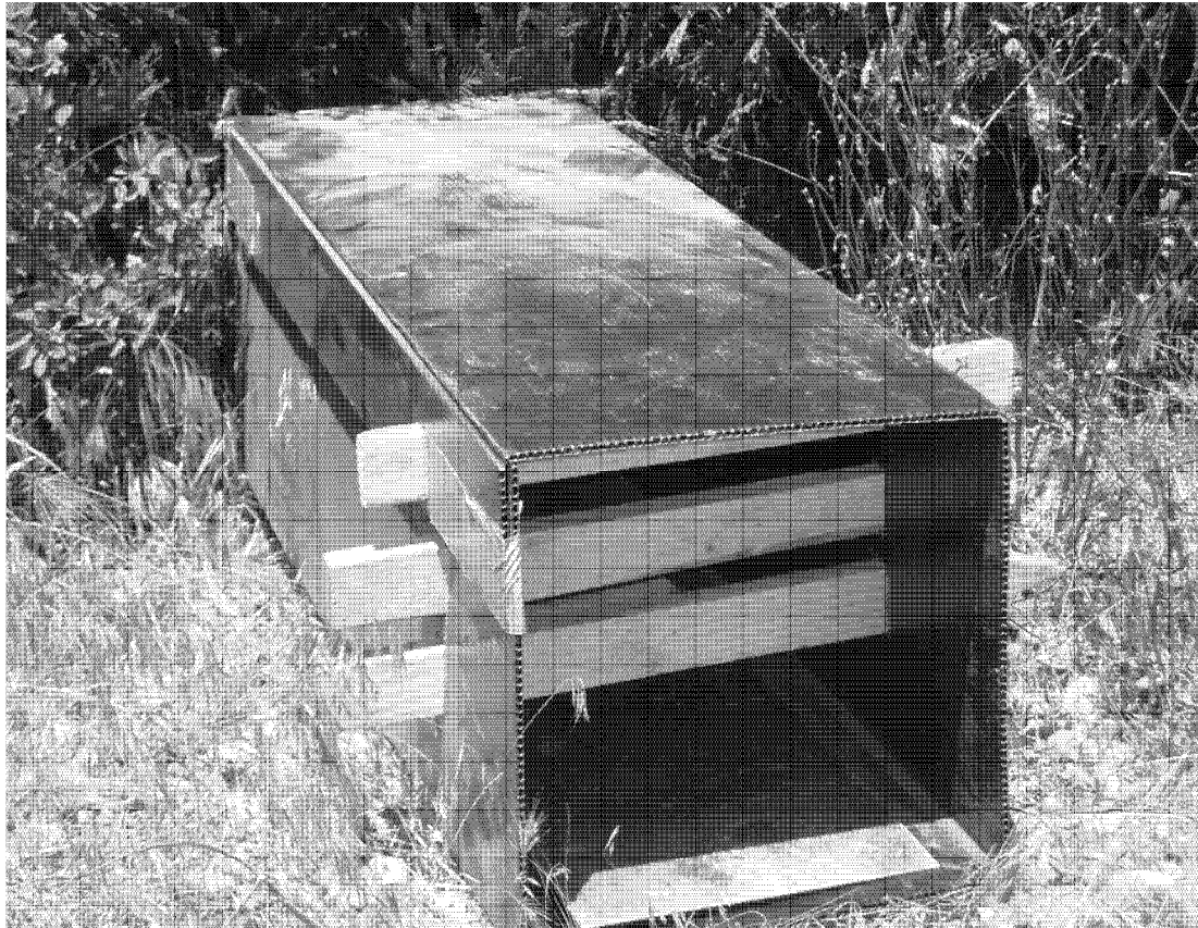
Figure 3: Coroplast fisher bait tunnel showing wooden slats at entry and track plate in place on bottom of tunnel interior. The bottom slat has a gluestrip underneath to collect hairs from mammals that enter the tunnel (photo by J.S. Yaeger, US Fish and Wildlife Service).
