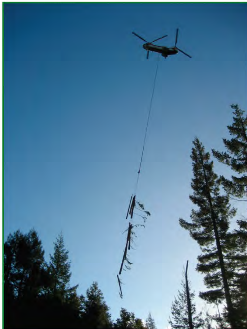
Figure 8.17. Vertol helicopter (10,000 lbs maximum external load) yarding in a fuel reduction thinning.
