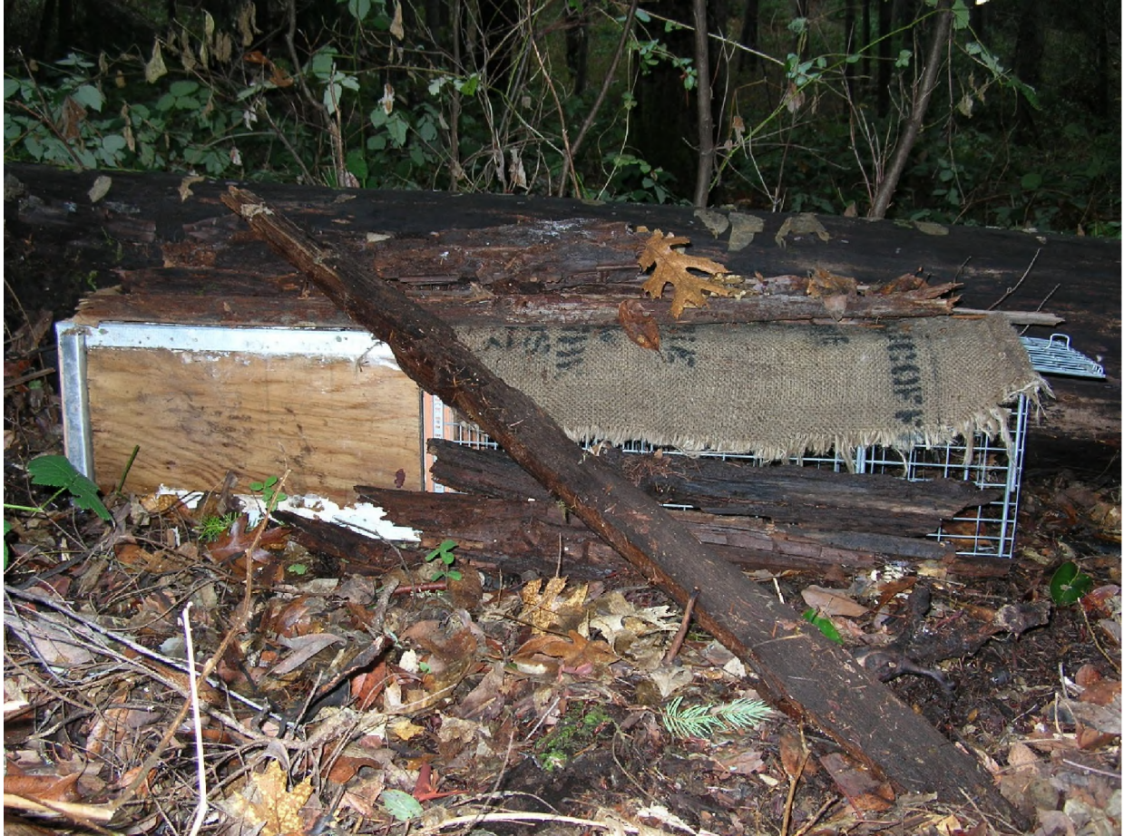
Figure 2. Tomahawk live traps (model 207, Tomahawk Live Trap Company, Tomahawk, Wisconsin, USA) baited with chicken legs and modified with a plywood cubby box to capture fishers.
