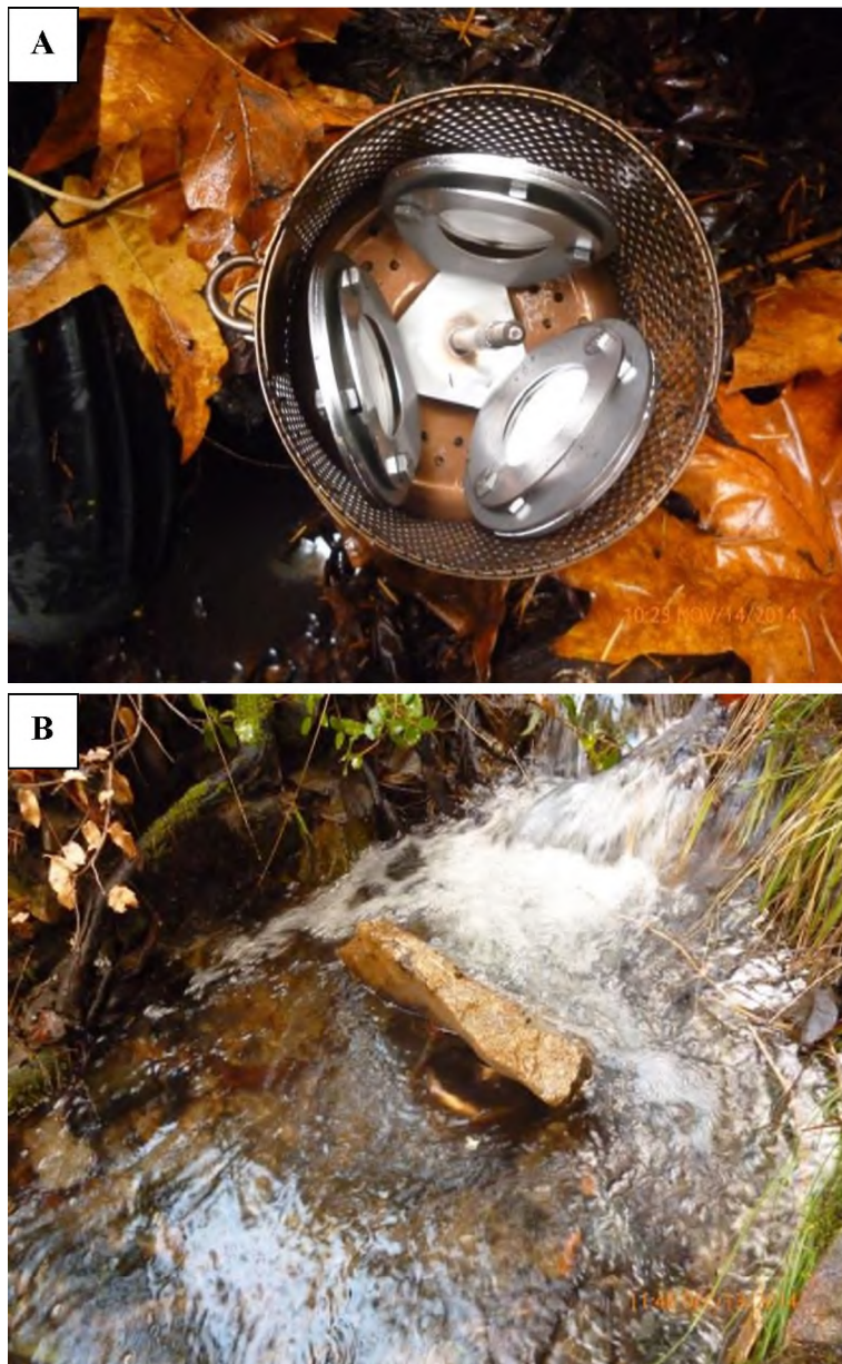
Figure 2. Examples of Polar Organic Chemical Integrative Samplers (POCIS) that were utilized to monitor water contamination by either polar or hydrophilic water soluble organic chemicals. POCIS units were placed in the streams immediately below trespass marijuana cultivation sites on Public Lands during the 2014-2015 season.
