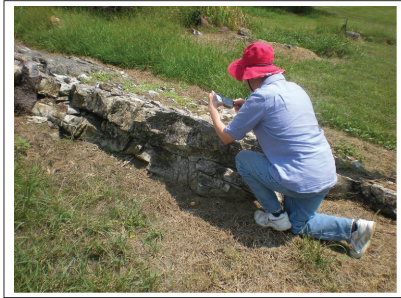
Figure 1.0.1-2 – Bedrock exposure near MP 194.3, showing the bedding planes parallel to the tilt of the bedrock and fractures perpendicular to the bedding planes.
