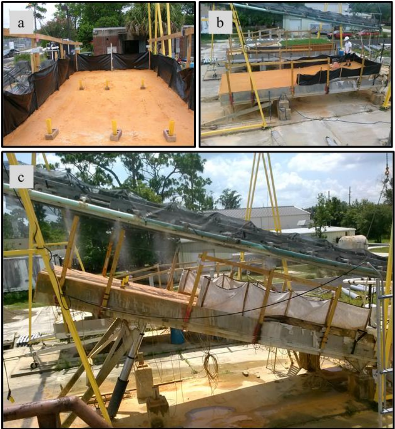
FIGURE 6 TEST BED SETUP (A) WOVEN FABRIC, RAIN GAGES, AND METER STICK INSTALLED, (B) TEST BED COMPACTION, (C) RAINFALL SIMULATOR AND TILTED TEST BED WITH NONWOVEN FABRIC INSTALLED
