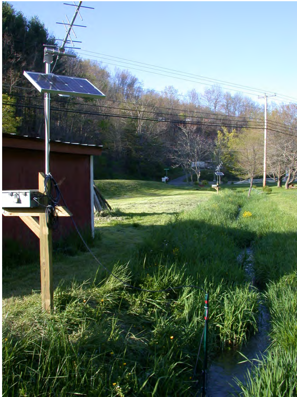
Figure 5. Water-quality monitors located on the unnamed tributary to Indian Creek, Tazewell County, Virginia. The monitoring station located in the foreground is the downstream monitor (Station number 03520980). The monitoring station in the background is the upstream monitor (Station number 03520981).
