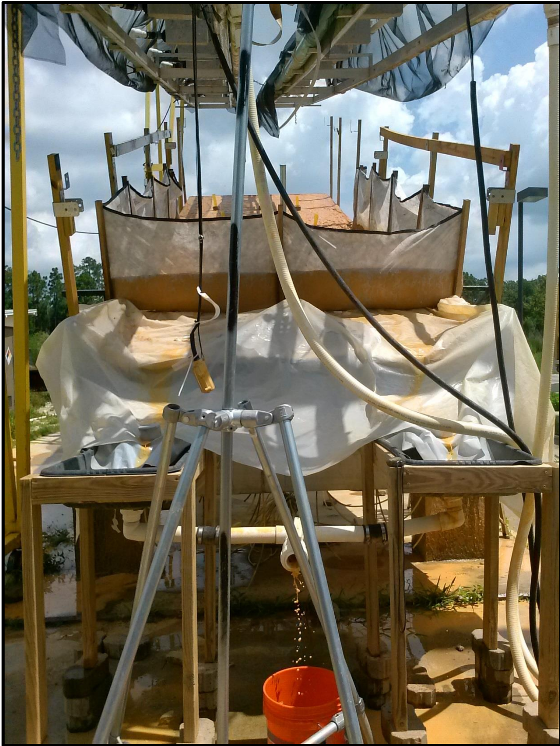
FIGURE 8 FIELD SCALE TESTING: DOWNSTREAM COLLECTION SYSTEM
