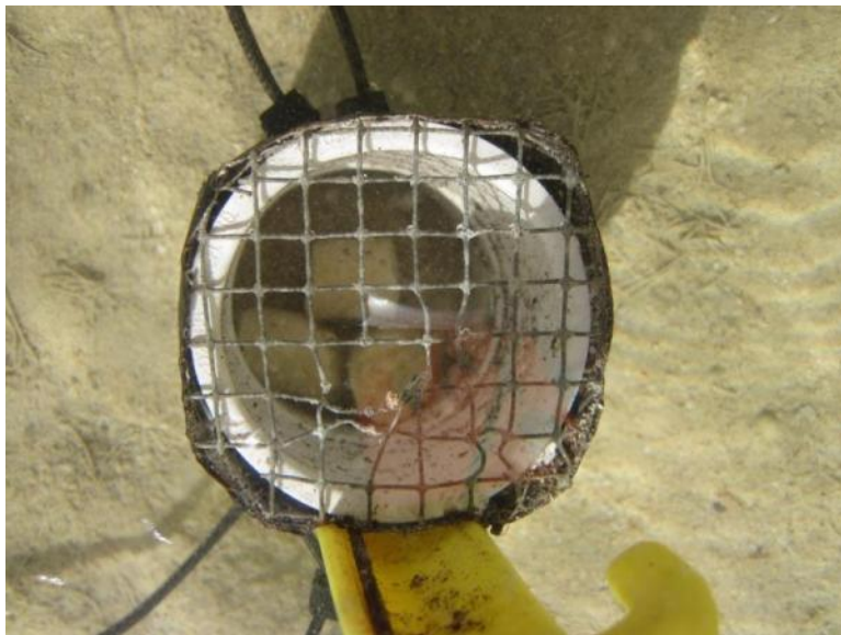
Figure 5: Placebo bait pellets inside the PVC exclusion cage with mesh top (yellow stake visible).
