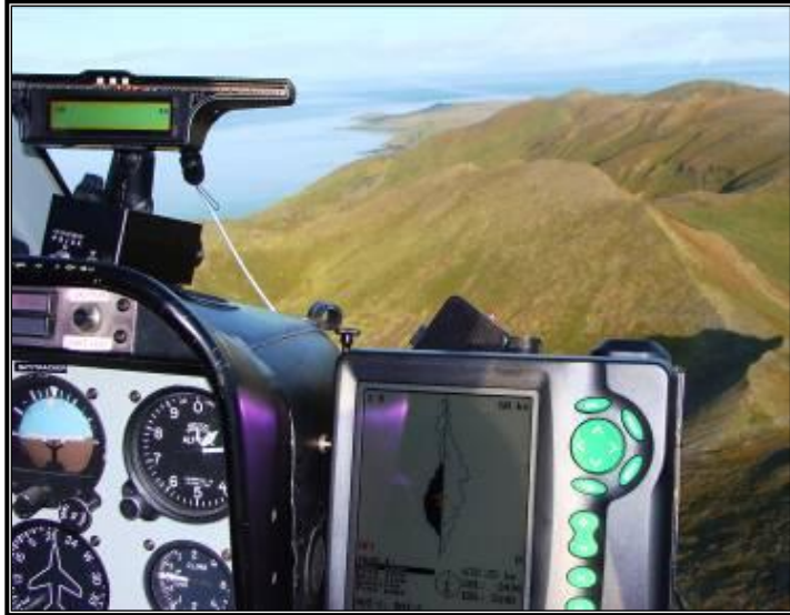
1 2 Figure 2.4. Onboard TracMap GPS used by a helicopter pilot to 3 monitor and guide the aerial bait broadcast at Rat Island, 2008.
