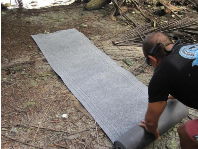
Figure 10: The noose carpet stretched across North Road on Cooper Island in an area where curlews are frequently observed. Hundreds of monofilament nooses (20 lb test) are incorporated into the carpet.
