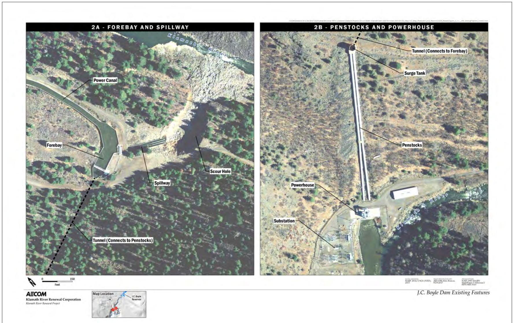
Figure A-3. J.C. Boyle Dam Forebay, Spillway, Penstock, and Powerhouse in Proposed Action
