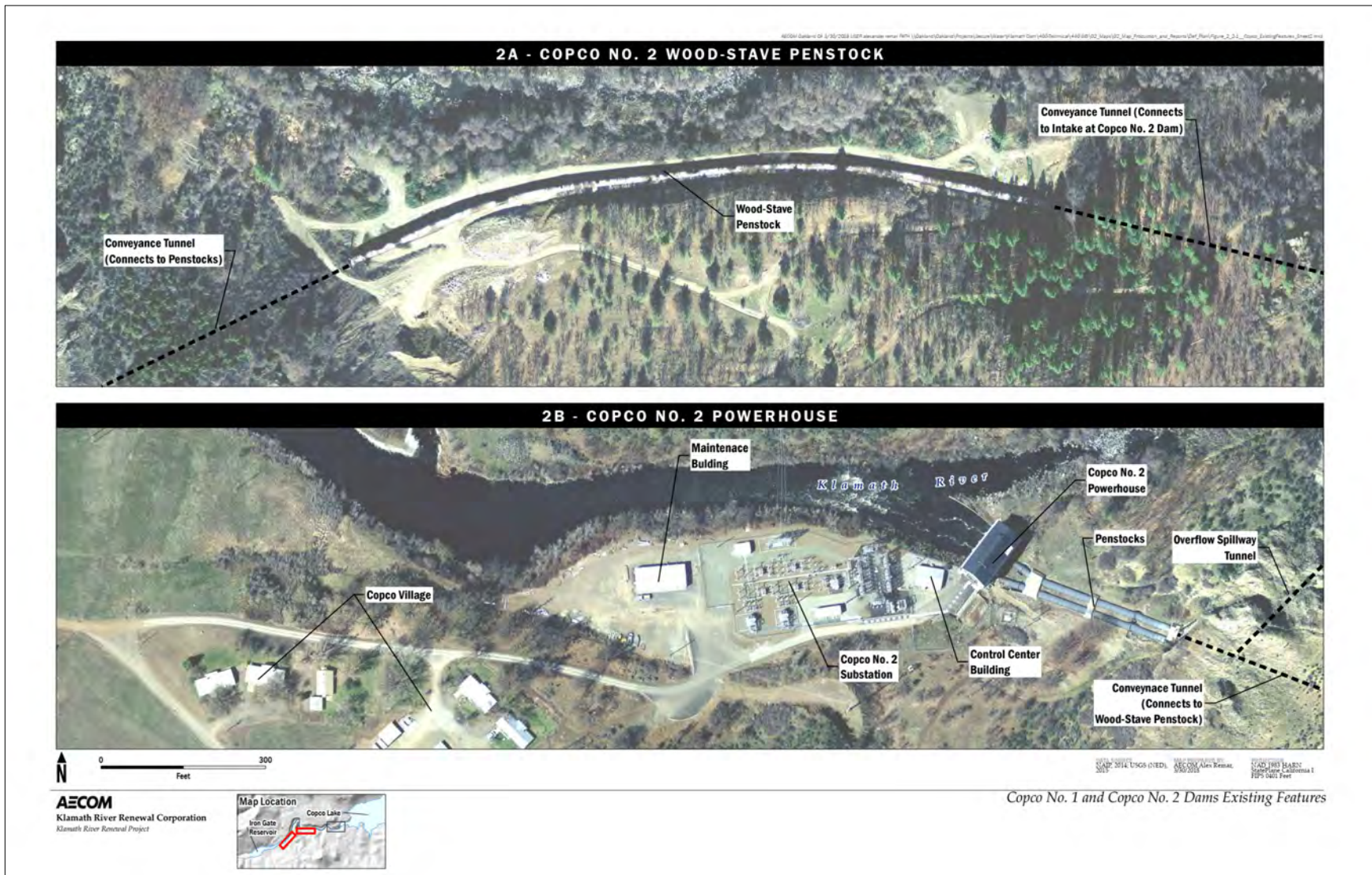
Figure A-6. Copco No. 2 Wood Stave Penstock and Powerhouse in Proposed Action
