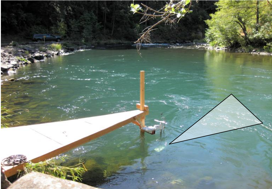
Figure 7. Scaffolding fabricated below the White Salmon River weir with the deployment bracket and DIDSON camera attached. The shaded triangle depicts the area being imaged by the DIDSON camera. The scaffolding was located approximately 18 feet downstream of the weir.
