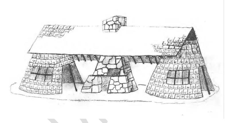
Concept Drawing for Alternative C – Retain conical base but remove cone tops and open up front and back windows.
