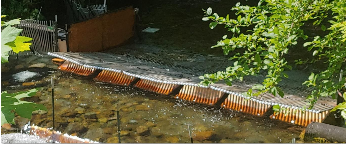
Figure 3. Photo depicting the aluminum picket leads, resistance board weir panels, video chute and camera chamber deployed in Cougar Creek.
