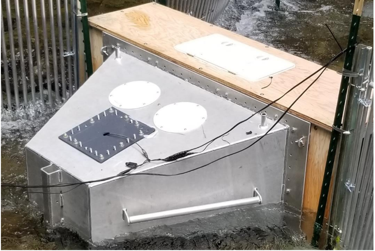
Figure 4. Photo depicting the camera chamber (left) and video chute (right).
